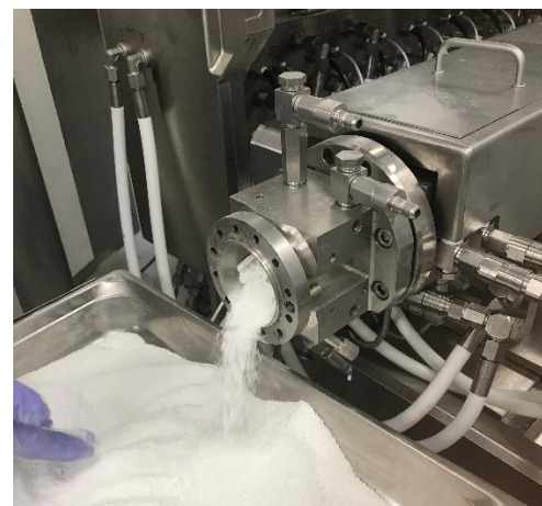
Figure 7. Granules prepared from HME.
