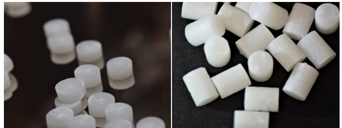
Figure 6. Cut rods prepared from HME.
