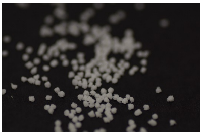
Figure 5. Micropellets prepared from HME.
