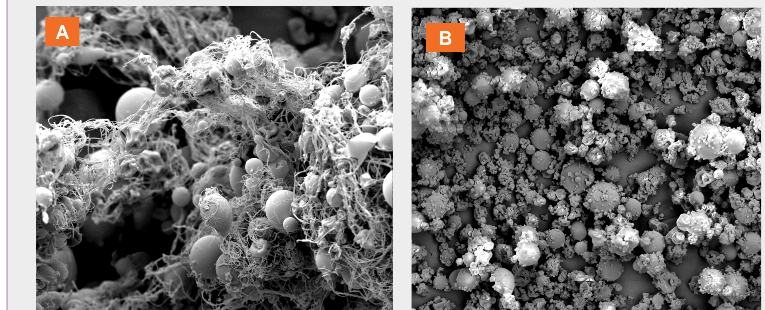
Figure 4. SEM images (1500 X magnification) of 100% EUDRAGIT® L 100 SDD, sprayed from 90:10 Acetone: Water at (A) 7% (w/w) total solids, inlet temperature of 102°C, atomization pressure 1 bar and spray rate 10 ml/min and (B) 3% (w/w) total solids, inlet temperature of 137°C, atomization pressure 1 bar, and spray rate 22.1 ml/min
